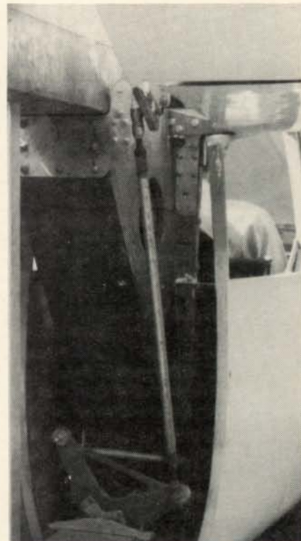
The rocker arm at bottom, located just forward of the mounting pad for the engine, is connected by torque tube to the stick mixer. Lateral control movements translate into direct aileron drive at inboard end through vertical pushrod, eliminating internal wing passages.
