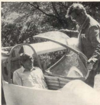
By golly, it fits! Designer Irv Culver positions the Windrose canopy over a happy Jim Maupin. The flat-bend plastic sheet is capped by a small molded sheet glued to the top section, but is basically a single-curvature canopy. Plenty of headroom has been provided.
